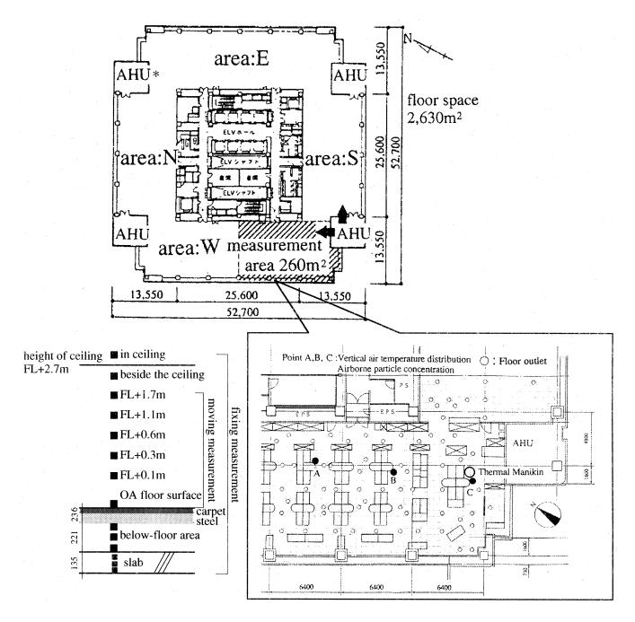
Figure 2 Floor plan and measured areas with floor outlet layout (plan) on the underfloor air-conditioning floor and vertical temperature measurement points (\*AHU is air-handling unit).
