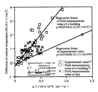
**Figure 6** Relationship between  $\Delta T/Q^2$  and difference in vertical temperatures.
