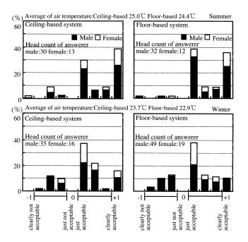
Figure 9 Results of acceptability for thermal sensation.
