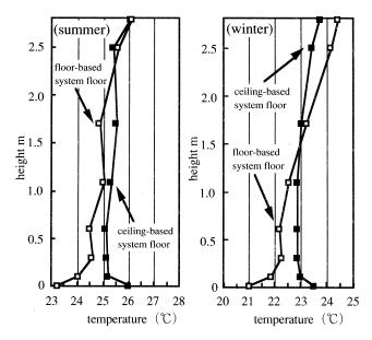
Figure 5 Vertical air temperature distribution.
