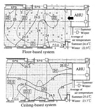
Figure 4 Horizontal distribution of air temperature at FL + 1.1 m.
