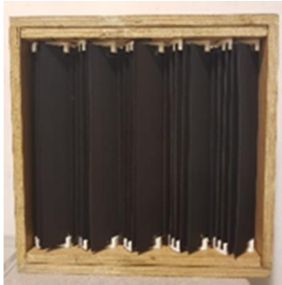
Biochar air filtration unit, with highly customizable dimensions and shape for different air duct systems
